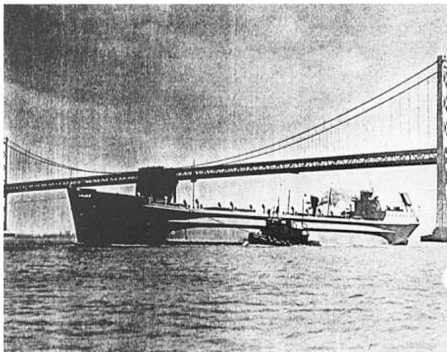
Figure # 1 General view - Dry cargo lightweight concrete ship, World War II
